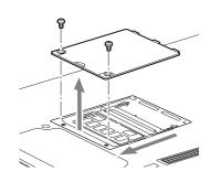
Figure 4-7. Opening the Memory Upgrade Compartment
